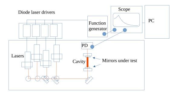
There are many variations for setting up a ringdown system, mostly determined by the lasers and wavelengths that are needed. The version shown here uses diode lasers, with fast electronic switching, which is low in cost and easy to use. Some beam shaping lenses are not shown here.
